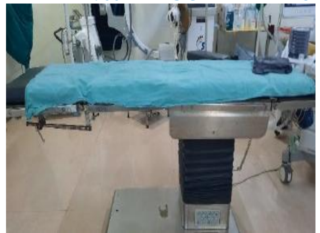
OPERATION THEATRE TABLE - C ARM COMPATIBLE ELECTRIC FUNCTION
