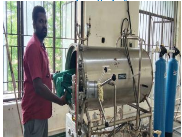
Horizontal cylindrical semi-automatic single door high pressure steam sterilizer
